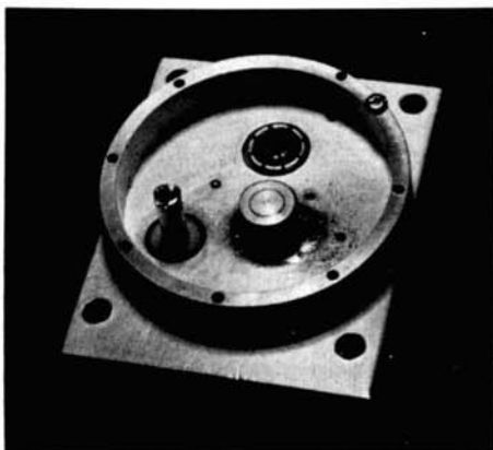
Inside view of the cathode partition and cavity assembly before it is attached to the plate assembly.
