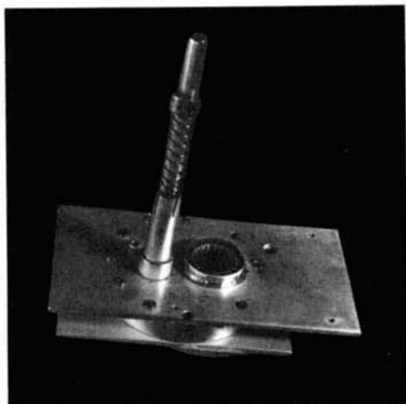
Plate assembly before installation of the cathode cavity.
